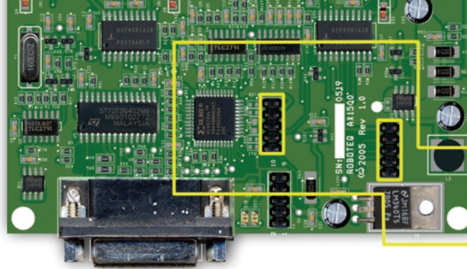
FIGURE 38. Position of Encoder Module on Controller's main board
